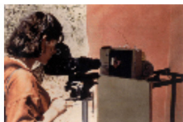
Figure 4.1 The photographic equipment in use, showing the vertical black backdrop against which the flowers, vegetation and grey scale are photographed, and the tripod-mounted camera with cable shutter-release, lens, filter holder, and filter in place.
