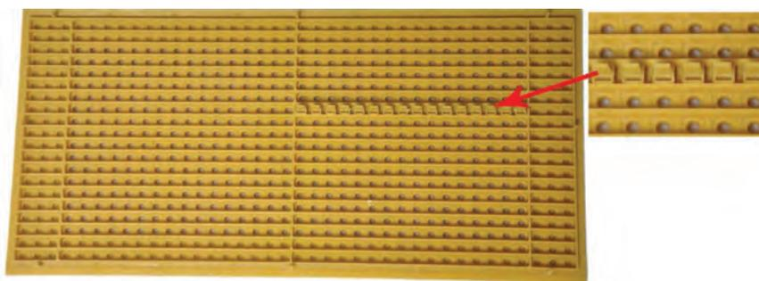
Fig 2. The back of the special plastic comb foundation (The hollow cell base on the back of the comb foundation can be match with the supporting larva device)
